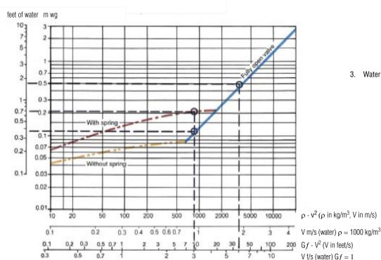
Water Flow velocity 6 ft/s and valve size 4".
