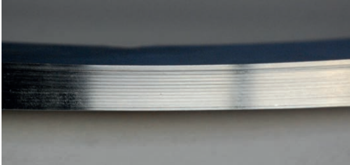
All metal lamination typically for wet steam applications
